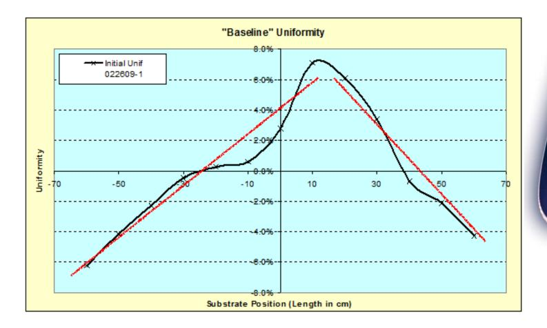
The dashed red lines show we have 2 slopes over the entire length. Both towards the center of the magnet array. We will add spacers and retest!
