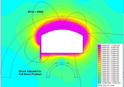
Depending on the size of the uniformity anomaly, shunts may be used on one or both sides of the magnet array. <u>Uniformity Optimization for Rotating Cylindrical Magnetrons</u> Uniformity Adjustment – A Working Example:
