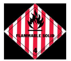
Hazard Class:4.1 Flammable solidsPacking Group:IIIUN Number:UN3089Proper Shipping Name:Metal powders, flammable, n.o.s. (Bismuth)
