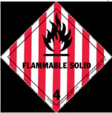
Hazard Class: 4.1 Flammable solids, self-reactive substances and solid desensitized explosives.
