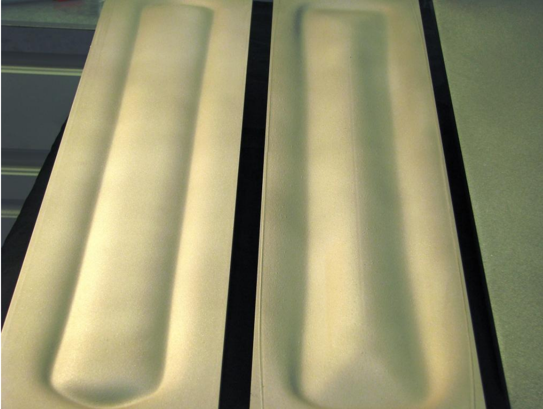
Figure 4: Erosion profile of target in old magnetron shown on left and erosion profile of target in new magnetron shown on right
