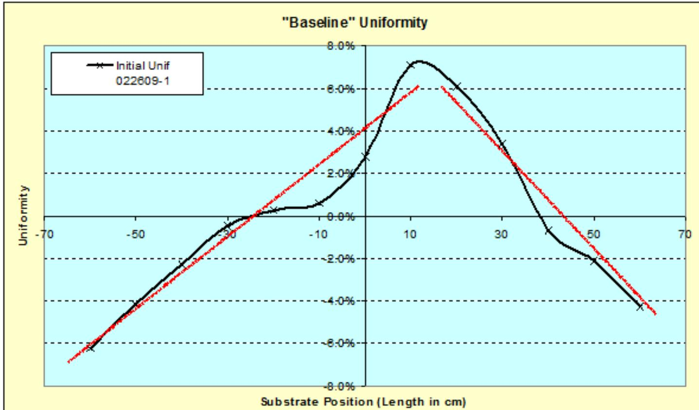
The dashed red lines show we have 2 slopes over the entire length. Both towards the center of the magnet array. We will add spacers and retest!
