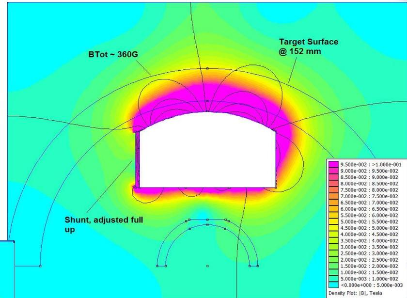
Depending on the size of the uniformity anomaly, shunts may be used on one or both sides of the magnet array.
