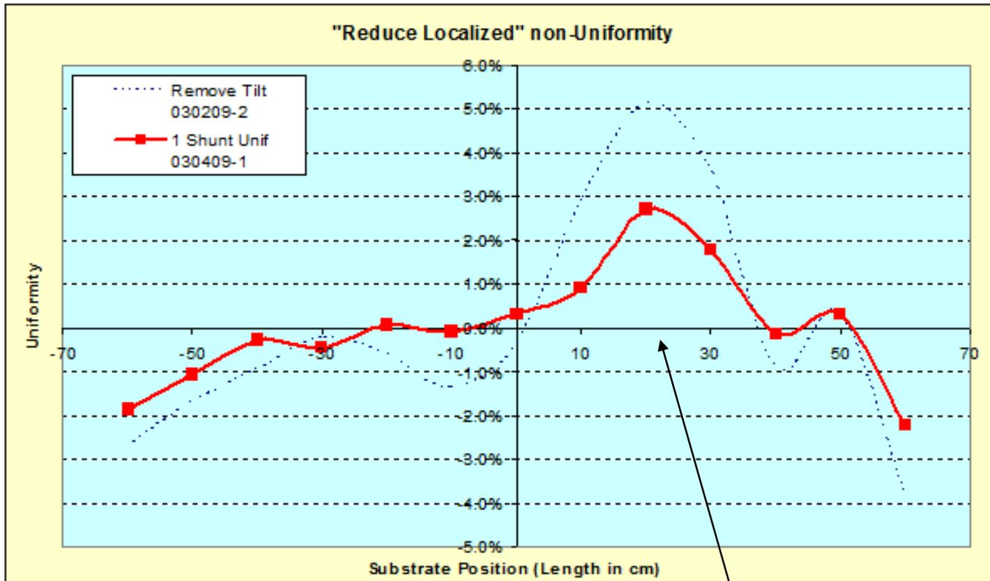
The addition of a single shunt brought the total uniformity in the correct direction but was not strong enough. Add 2<sup>nd</sup> shunt to other side of magnet array!
