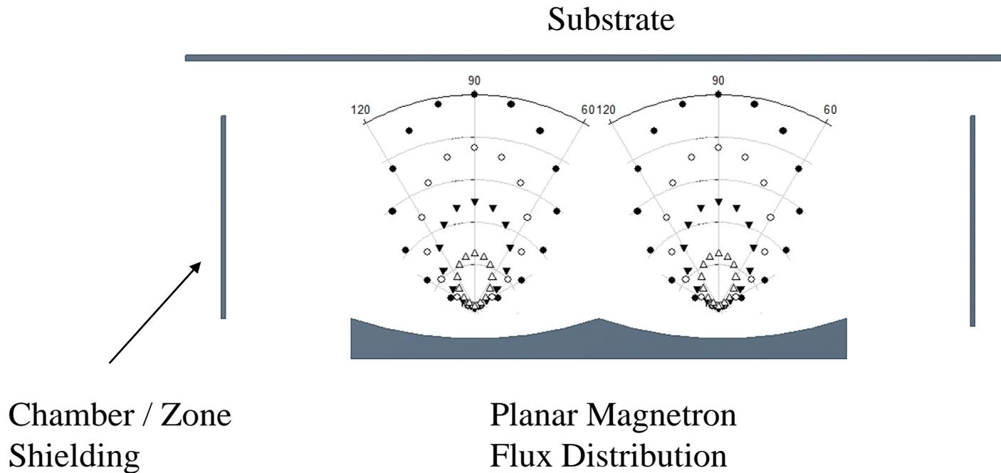
The “normal” orientation of the material flux to the substrate helps to minimize the amount of debris migrating to the sputter shields
