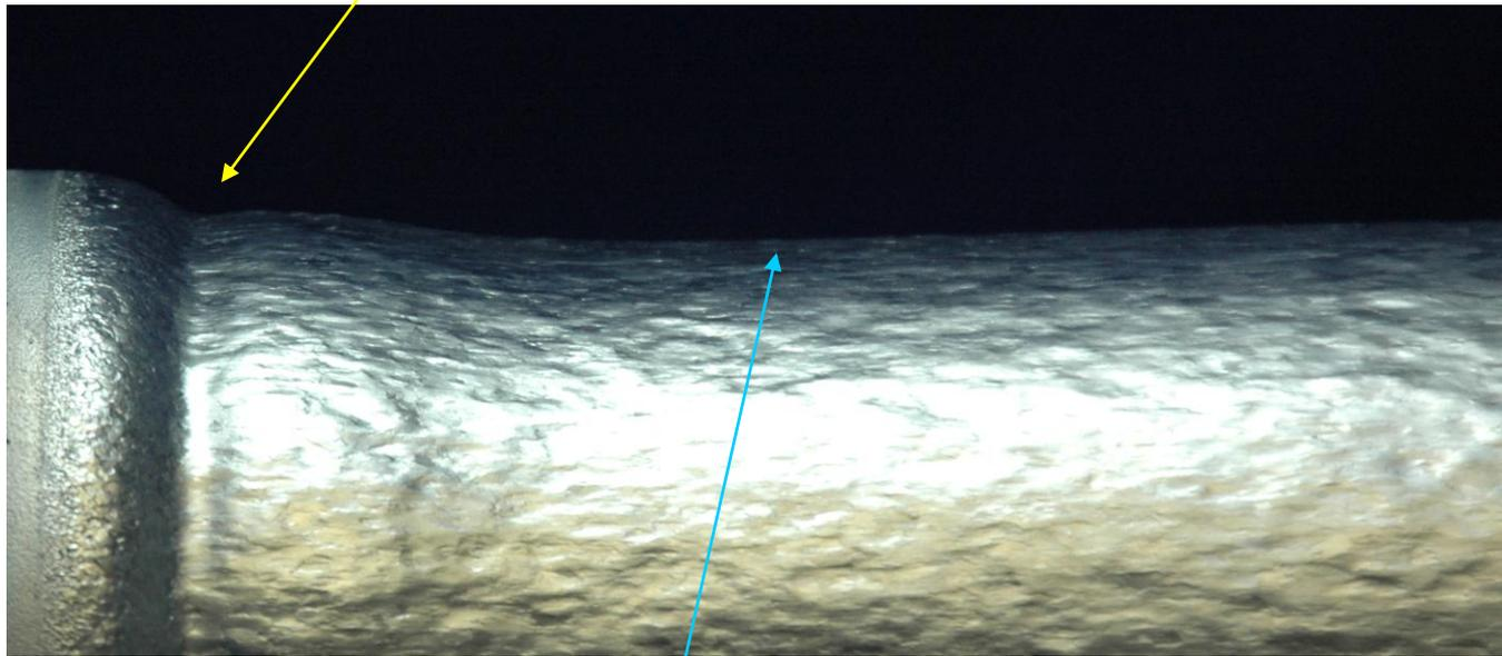
Deepest Erosion is along the length of the target surface
