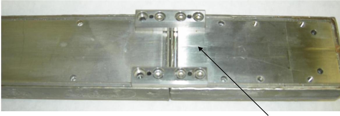
Addition of Spacers to Adjust Magnet Array to Target Surface Distance
