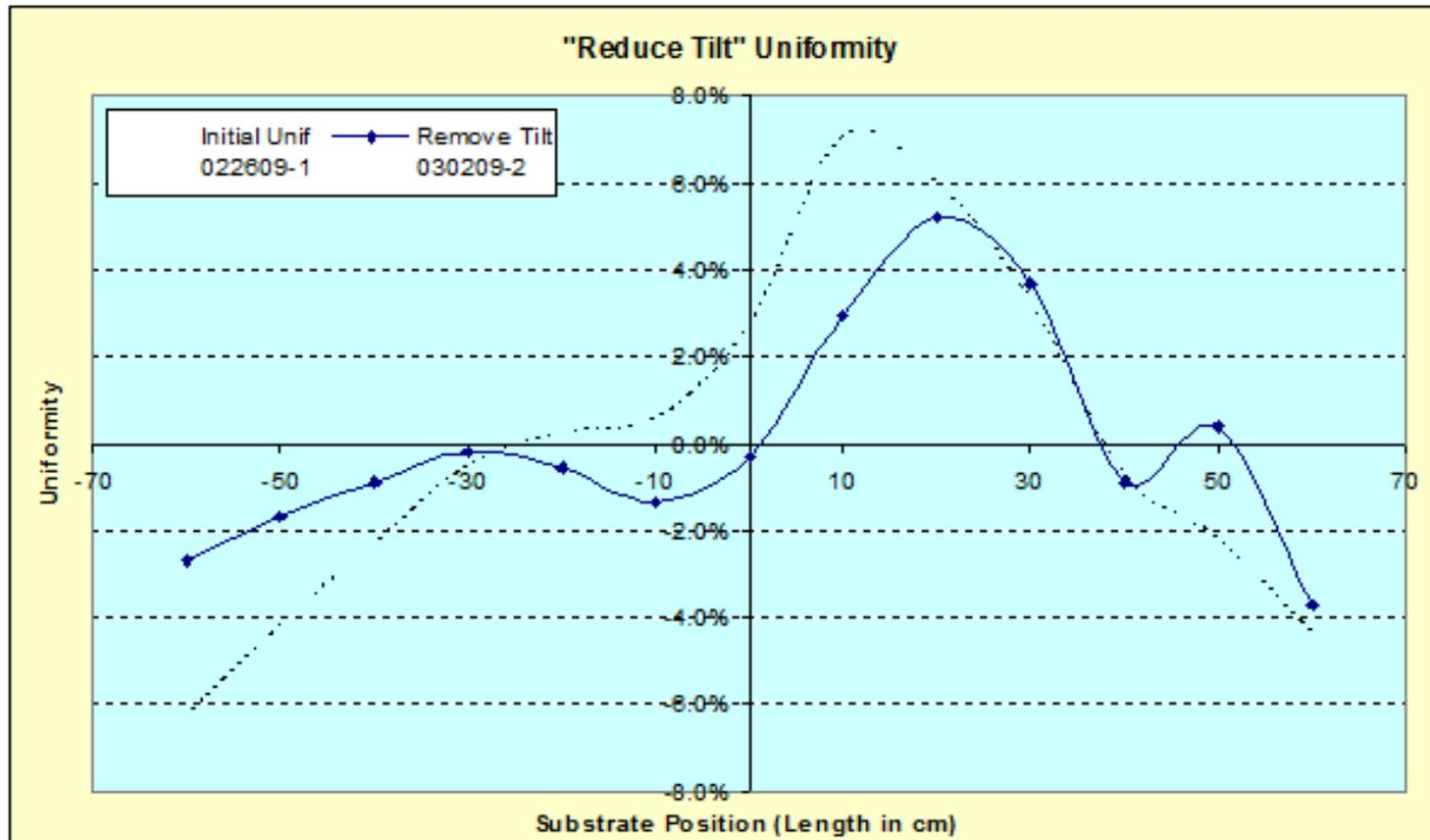
At this point we can either try further adjustment to the tilt, or, try to remove the “local” non-uniformity
