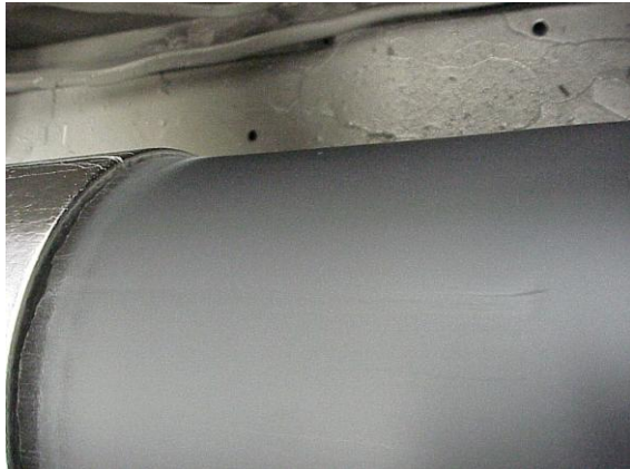
After 7 days of testing, 24 hours of operation per day, the ITO cylinder is still clean of any nodules or signs of cracking. This last day of test was conducted at 2.5X power
