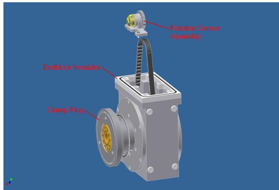
Also, the Rotation Sensor Assembly needs to go back on using the (2) #8-32 x 0.500" SHCS.
