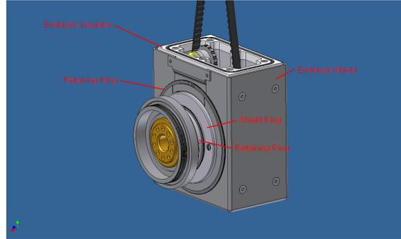
**Note:** All o-rings in the Endblock and Target assemblies should be cleaned as necessary and lubricated with vacuum compatible grease.
