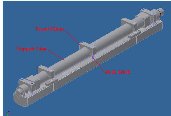
2. Insert the necessary shims as determined by analyzing the uniformity data and replace the Target Clamps and SHCS.
