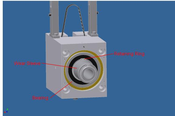
7. With the Shaft Assembly removed from the Drive Block, the Belt can be set aside. Next, loosen the set screw in the Wear Sleeve. The Retaining Ring on the end can be taken off, then slide the Wear Sleeve off and take the other Retaining Ring off of the Drive Shaft. Now loosen the set screw in the Drive Pulley and slide it and the Brush Housing off of the Drive Shaft.
