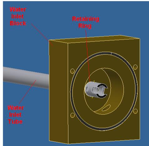
Prior to reassembly the face seal o-ring grooves should be cleaned and the o-rings should be cleaned/inspected for replacement.
