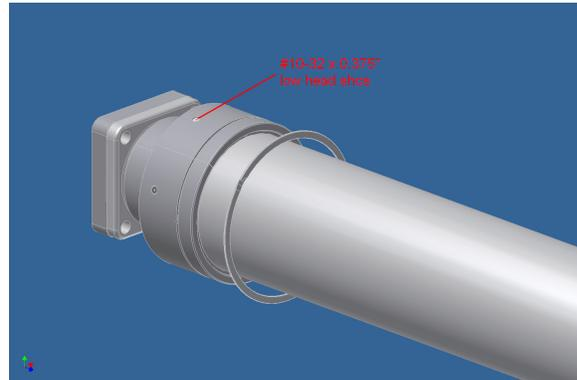
4. With the mounting screws removed, the Debris Shield can be separated and fully detached from the Target Assembly. For separating the Debris Shields, pull each side straight away from the other so as not to bend the guide pins. These pins align and position each side to one another. At this time the Debris Shields can be grit blasted for material removal. Many users have spare replacement Debris Shields Assemblies that can be pre-cleaned and readily installed to reduce system "down-time."
