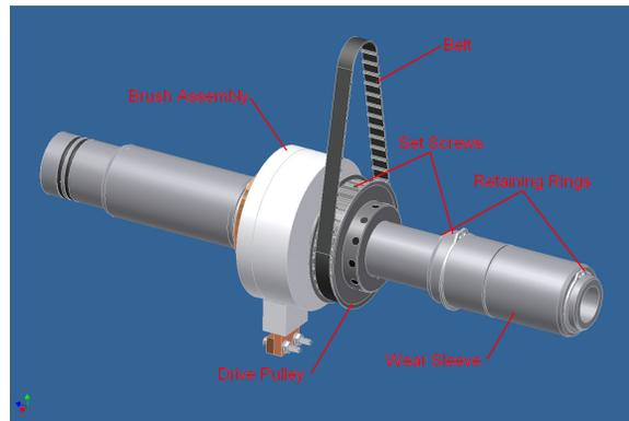
8. Remove the (4) #8-32 x 0.500" SHCS so the Brush Assembly can be opened up.
