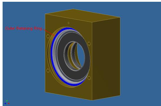
**NOTE:** Make sure to have the flat face of the seals facing the front of the housing (side with dowel pin hole) and the cupped side facing the water return hole.
