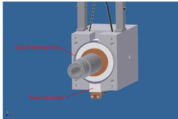
5. On the back of the drive assembly, the spiral retaining ring and Drive Insulator Cap should be taken off.
