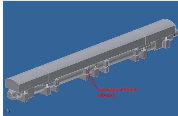
5. Install the shunts on the mounts at the desired height as determined by the uniformity data.
