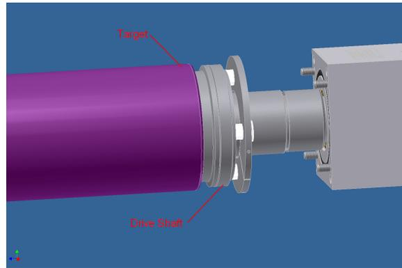
On a non-bonded assembly, the Lifting collar can now be removed. Notice the gap in between the wave spring and Target Retaining Ring, this is where the Target Clamp will be installed.
