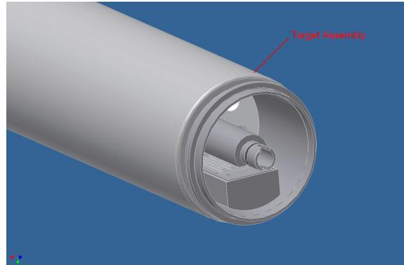
5. The Magnet Pack and Support Tube can now be pulled out from inside the Target.
