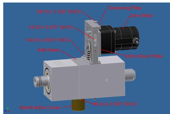
**NOTE:** When reattaching the motor, lift it up to remove the slack in the belt and place the 3/8-16 x 1.500" SHCS through the Tensioning Plate and tighten it into the Motor Mount Plate until there is very little slack in the belt (it should appear tight at rest, but deflect about 1/2" to 1" when pressed on by hand). As long as the belt doesn't slip while rotating the target, it is tight enough.
