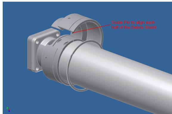
5. For reassembly of the debris shields onto the target assembly, reverse steps 2-4 of the Debris Shield Removal procedure above. To check successful reassembly, use an ohm-meter to check conductivity between the Debris Shield and the Target surface. This should be an OPEN (no contact) circuit. Check each Debris Shield also to the chamber or system ground. This also should be OPEN circuit.
