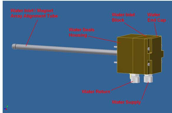
**NOTE:** All of the seals and o-rings in the Water Housing are only sealing between water and atmosphere. Because there is no exposure to vacuum the best lubrication to safely use is a marine grease. This lubricant is water compatible and will offer a longer service life than vacuum compatible or standard grease.
