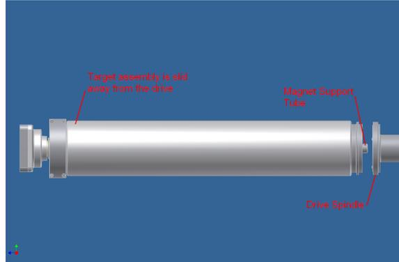
4. The Target Assembly should be moved to a cart or table in order to take the Magnet Pack out. With the Target out of the chamber, it is possible to drain any water that may be left inside of the Target.
