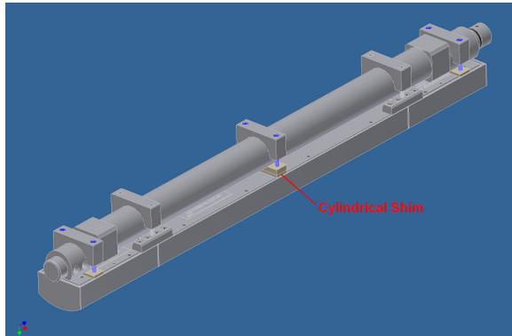
**NOTE:** For the “stepped” Magnet Support Tube design, an additional 0.250” shim will need to be placed along the center section of the tube if it is not already there. The Magnet Kit is generally designed to be shimmed no more than 0.125” from the Support Tube.
