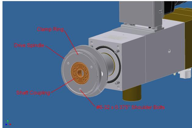
4. The Drive Spindle is held on with (8) #12-24 x 0.750" shcs. Once these screws are removed, the spindle can be pulled off of the Drive Shaft. It may be a tight fit because of the double radial o-ring seal between the spindle and the shaft.
