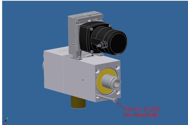
8. Before the cathode is attached to the chamber or flange, the o-ring seat, mating flange and sealing o-ring should be cleaned. The metal surfaces and the o-ring can be wiped clean using a lint-free wipe with a cleaning solvent. After cleaning, the o-ring can be lightly lubricated with vacuum compatible grease.
