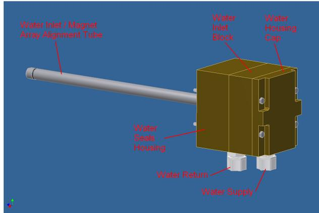
**NOTE:** The cooling water flow requirements of the cathode are 1 gallon per minute (GPM) for every 4 kW of cathode power. It could also be stated as 0.25 GPM per 1 kW of power. In metric units the requirement would be 1 liter per minute (LPM) for every 1 kW of cathode power. For example, you would need 3 GPM (or 12 LPM) if you were running 12 kW of power.
